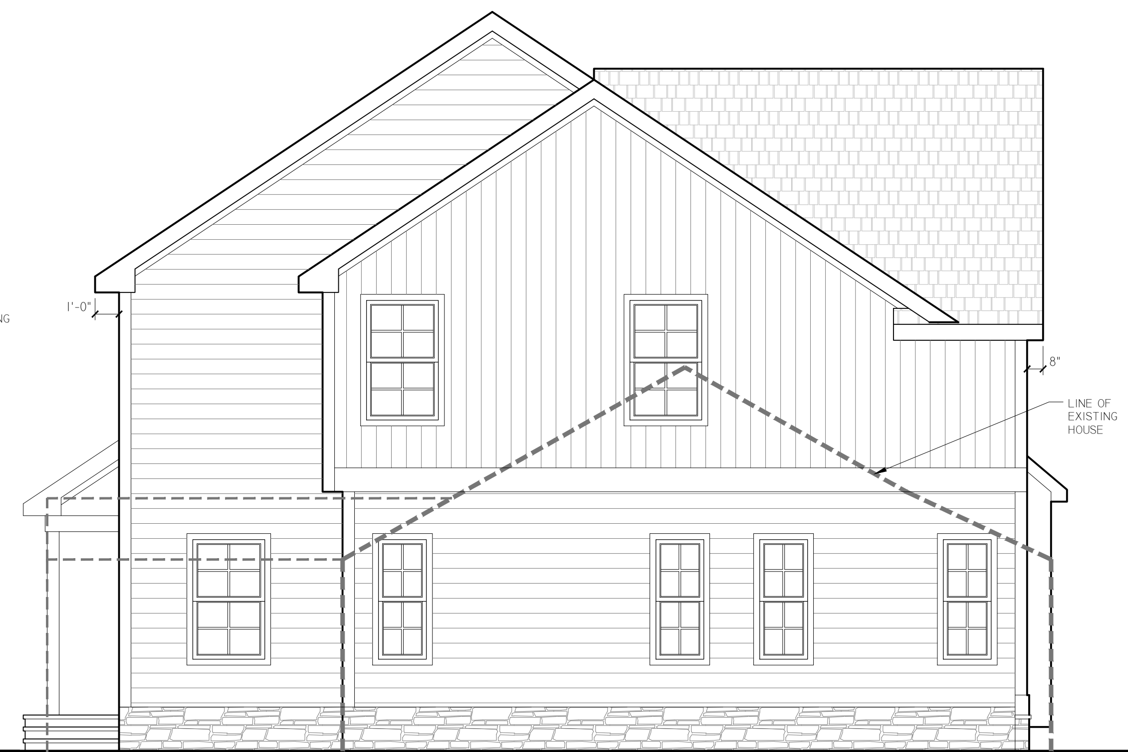
PROPOSED LEFT SIDE ELEVATION SCALE -- 1/4"=1'-0"
