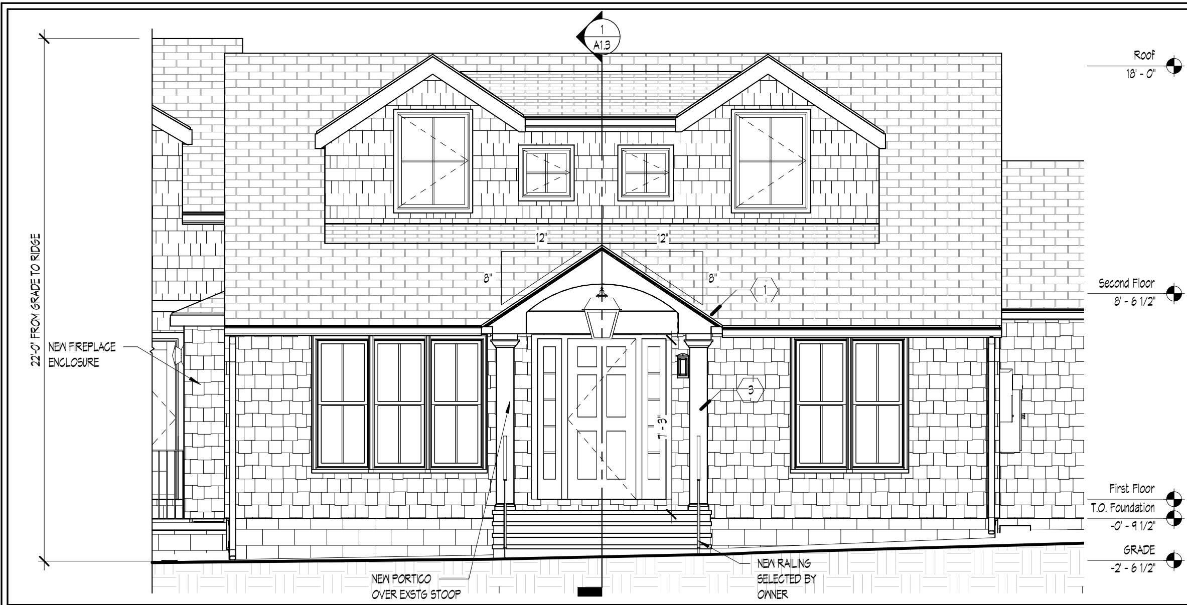
2 PARTIAL PORTICO ELEVATION 1/4" = 1'-0"
