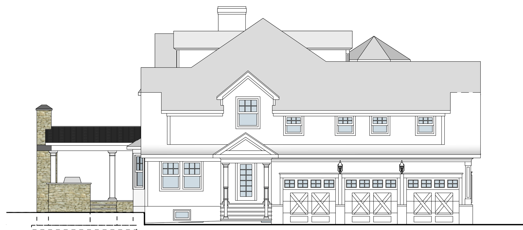
SIDE ELEVATION SCALE 1/8" = 1'-0"
