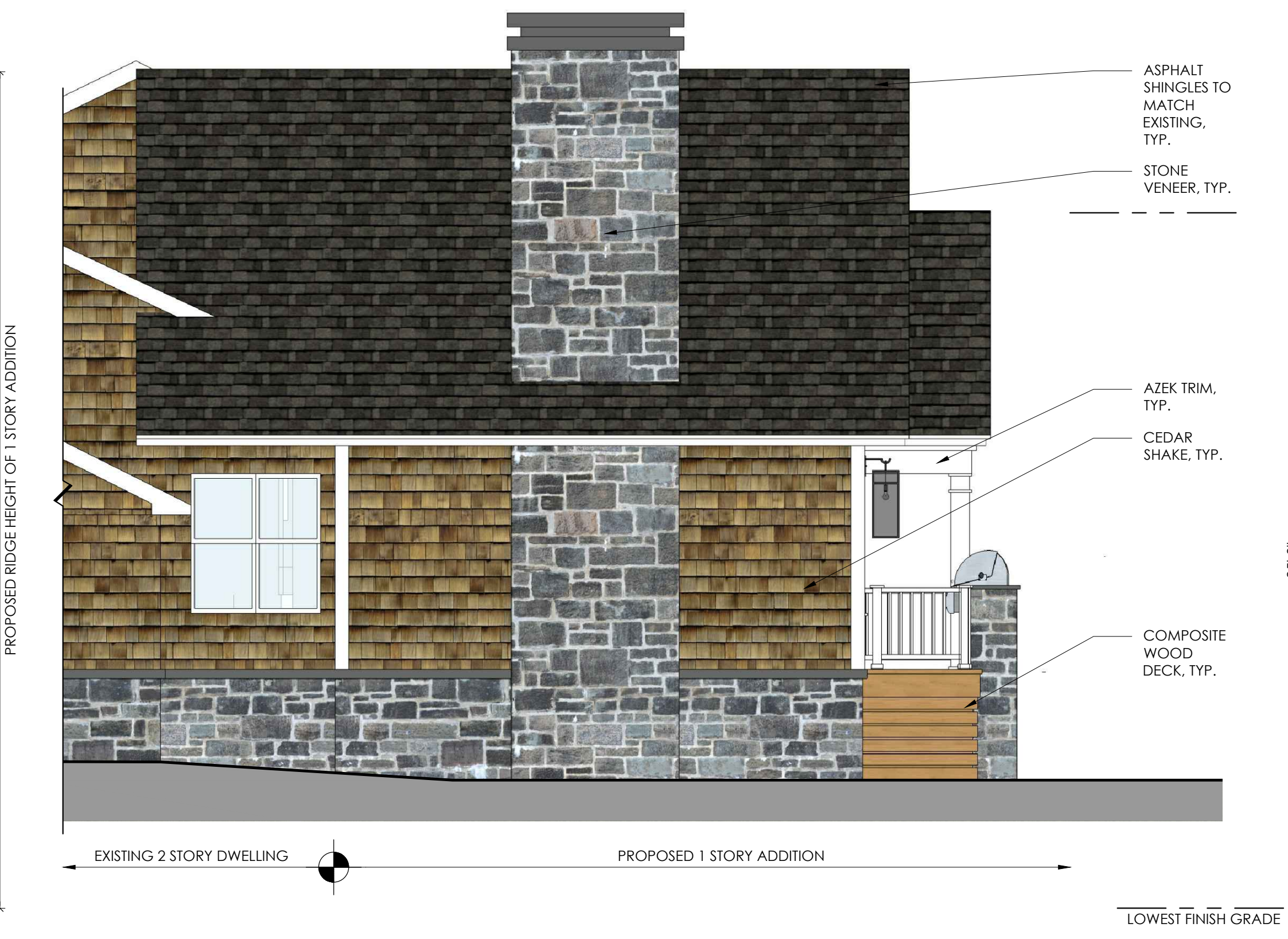
1 PARTIAL EXTERIOR ELEVATION: RIGHT
