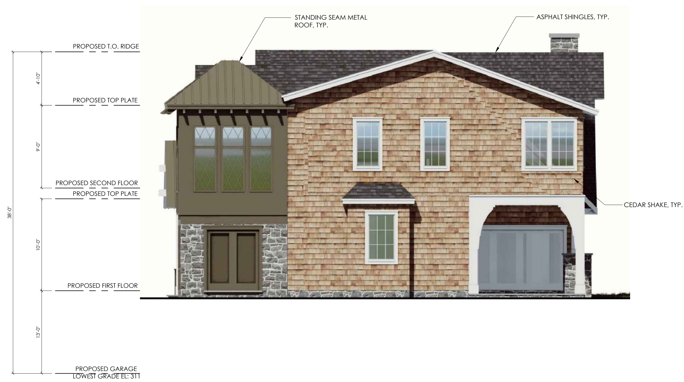
2 EXTERIOR ELEVATION: RIGHT
